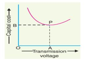
The **empirical formula** to find the economical transmission voltage between lines in a 3-phase ac system is :
