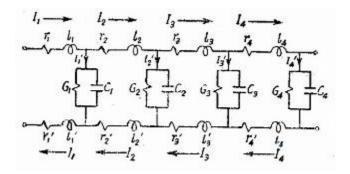
The same current flows through the upper and lower part of each section the resistance and inductance of both can be combined and the equivalent circuit of below fig. is obtained. Thus: R1 = r1 + r1', L1 = l1 + l1'......etc.
