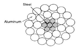
ACSR consists of a central core of steel strands surrounded by layers of aluminum strands. ACA R has a central core of higher- strength aluminum surrounded by layers of electrical- conductor grade aluminum.
